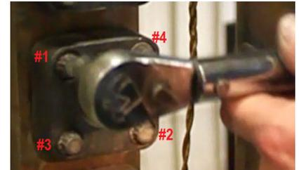
14. Re-install the illuminator and level display.
