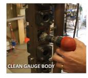
Clean each port in the gauge Body using a wire brush and wipe clean
